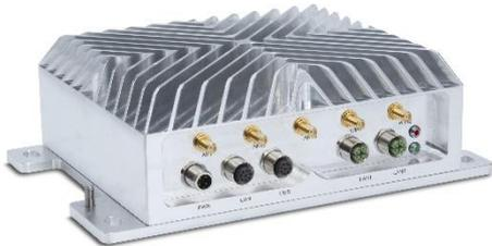
Our final Best in Show recipient, the AI Rugged Computer from Syslogic, provides a hardware base for AI edge applications under extreme conditions thanks to the use of Nvidia's TX2i
