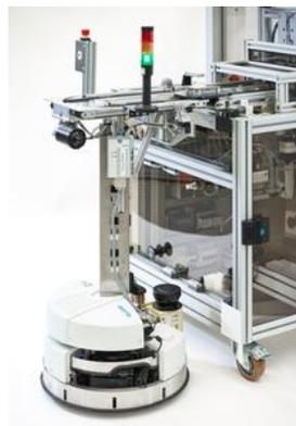
*Products can now be manufactured in different ways because of the use of the flexible transport system comprised of a robot platform as the central element as well as the conveyor belts in the modules. ©SmartFactory<sup>KL</sup> / C. Arnoldi*
