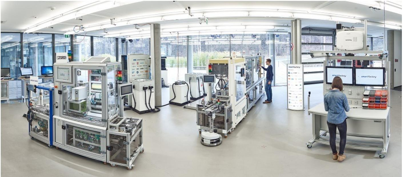
*The modules of the demonstration system of the SmartFactory<sup>KL</sup> partner group is distributed over three production islands to enable flexible production. ©SmartFactory<sup>KL</sup> / C. Arnoldi*
